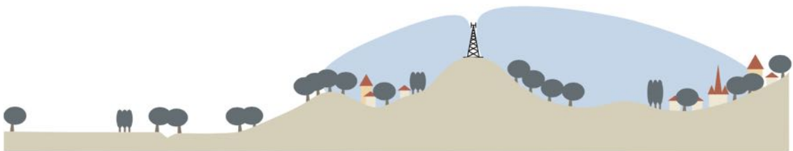
Figure 2 2 . Ideal elevated location for a mobile base station which allows for unobstructed signal travel
